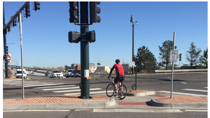
Most signalized intersections are equipped with pedestrian-actuated push buttons, and pedestrian signal heads that instruct pedestrians when it is appropriate to cross the intersection (Image: Church Ranch Blvd and 104th Ave).
