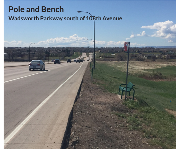
Benches at bus stops are an enhancement, but sidewalks should also be provided so those with disabilities can access the station
